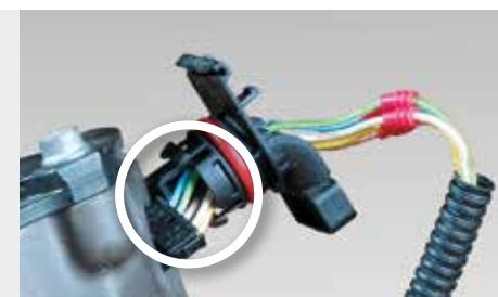
Faulty connector. The connector has snapped off.
