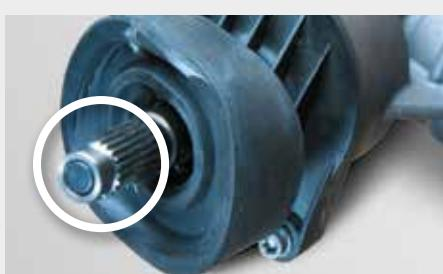
Missing protective cap. This can result in external parts, such as the spline drive, being damaged during transport.
