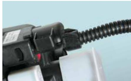
The protective caps removed from the new part must be applied to the used part for return. Seal all open holes!
