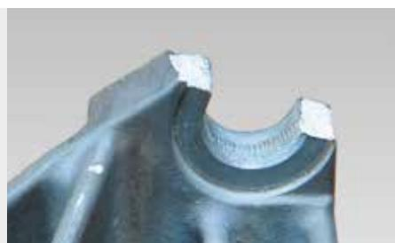
Damage caused by external use of force. A piece of the metal eye from the steering gear has broken off.
