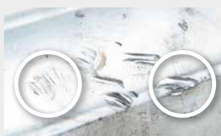
Body damaged by external use of force, with possible resultant damage to the electronics.
