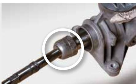
Track rods not removed. To ensure safe transport, the track rods must first be removed.
